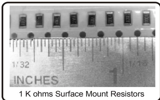
around the cylinder. Surface Mounts are available in much the same package sizes as the LEDs. The number of ohms is printed on the top side of the resistor.
