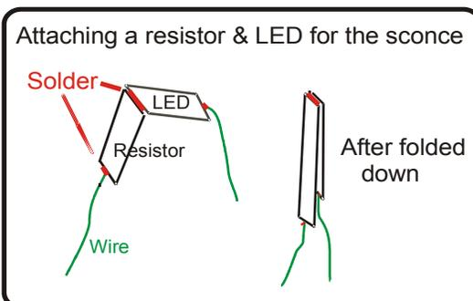
Then I place them on the tape so that the two ends without wire are next to each other and solder them. If they are going to fit into a very small space, then I place and solder them so that they are back to back without the wired ends touching. To ensure this distance, I usually use two different sizes of SMD. After the soldering is done, I insulate it with clear nail polish as a precaution against a short circuit.
