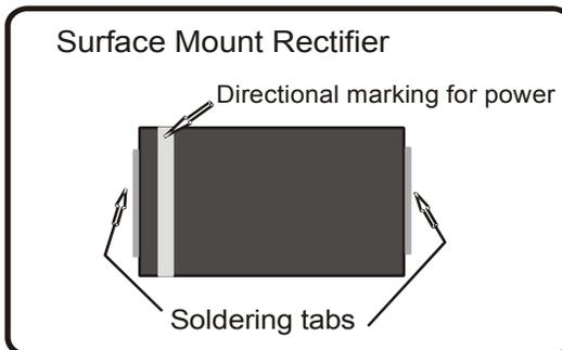
On my baby house boards, I have been using surface mounted "Fast Recovery 1A 50V" rectifiers. They are surface mounted on the lower right hand side of the board just above where the lead-in from the transformer comes in. If you are putting the rectifier in a doll house or room box circuit, using wiring or tape wiring, then the Axial rectifiers are better to use. Usually, only one rectifier is needed for our projects. One rectifier will work for about 75 LEDs.
