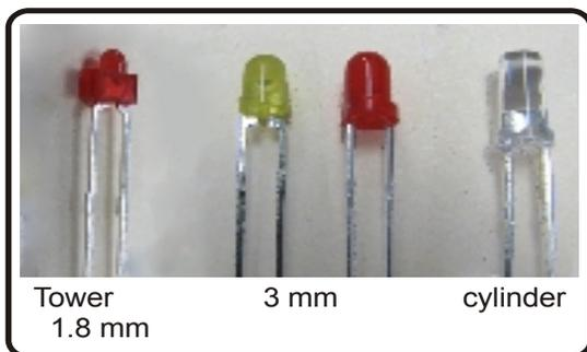
legs. One of the wires is shorter than the other wire. This is very important. As I described above, the electrons flow through the LED and set them up to glow. If the LED is not oriented in the correct direction, the electrons do not line up, but push away from each other. To get the light, the electricity must enter them at the correct end and exit at the other end. The longer leg is the anode (positive) and the shorter leg is the cathode (negative).
